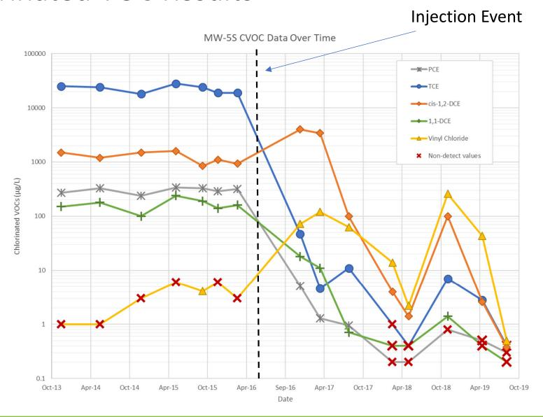
EOS 100 and ABC co-injected in a barrier (MW-5 is down gradient)
